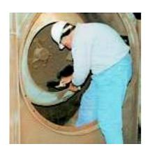
CERAMIC REBUILD PUTTY Highly advanced epoxy putty that provides suitably treated equipment with exceptional resistance to erosion, cavitation, corrosion and chemical attack. Repair or rebuild pumps, impellors, liners, valves, elbows and other components used in power plants, pulp and paper mills, and other industrial Kit Contents 1 kg applications.
