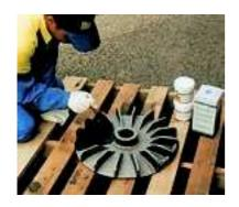
SYNTHETIC RUBBER PUTTY Liquid polyurethane that becomes a smooth trowellable paste upon mixing. Cures to a tough, flexible rubber that exhibits excellent wear and abrasion resistance. Suitable for use in lining and protecting equipment such as chutes, pumps, agitator blades, screens, and in the repair of existing rubber linings for abrasion resistance or noise abatement services.
